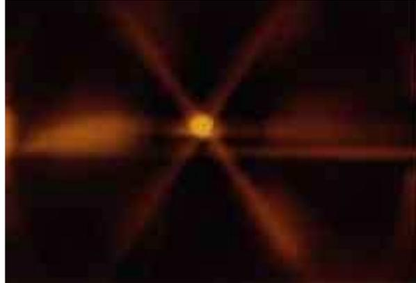
The image above shows sodium atoms (the bright spot in the center) trapped at the intersection of three orthogonal pairs of opposing laser beams. The trapping region is called “optical molasses” because the dissipative optical force resembles the viscous drag on a body moving through molasses.
